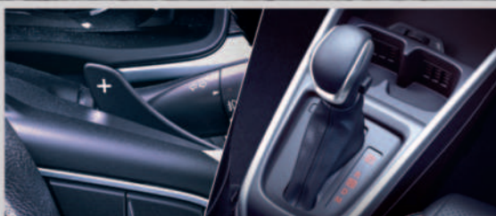
6-Speed Automatic Transmission with Paddle Shifters
